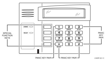
6160RF Keypad/Transceiver (front door removed)
